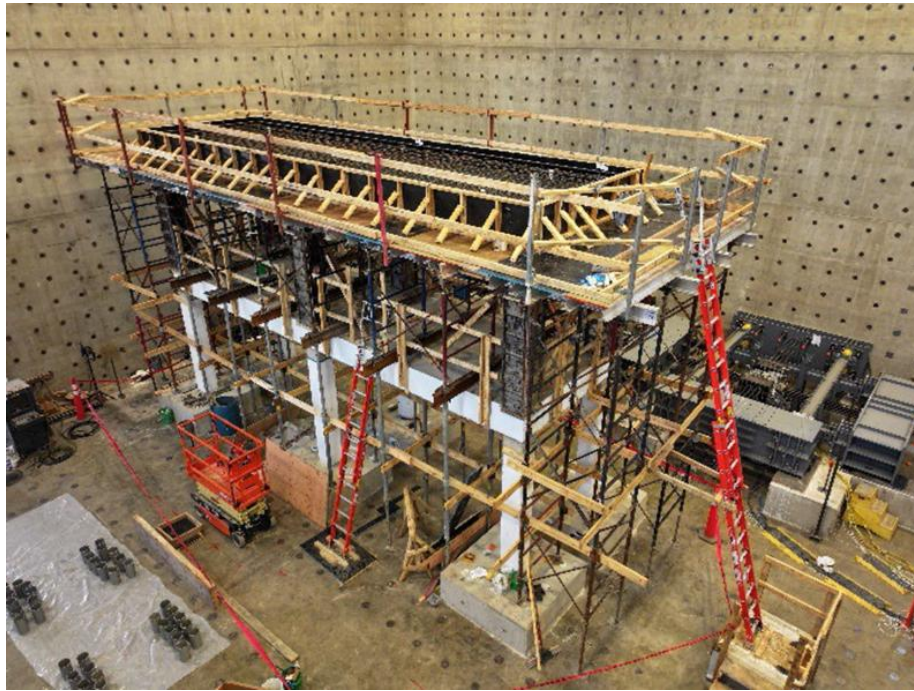
Fig. 24. Two blind competitions used for FEM model tuning and validation in Task 2.4, (left) prestressed RC girder from Swiss test, (right) experiment of full scale two-story RC frame from Purdue University.
