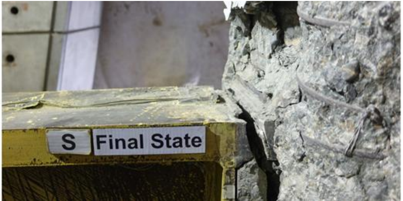
Fig. 23: Rupturing of the beam's flange (EJH specimen) during the experiment.
